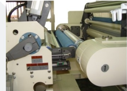
收料座 配備近接輪以做更佳捲取 Rewinder provided with near roller system Before rewind shaft for better rewind condition
