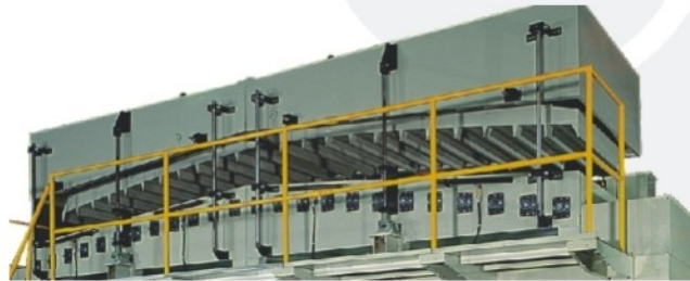
鋼製乾燥箱導輪, 研磨完成附驅動 All the guide roller in dryer made by steel Grinding finished and with driving
